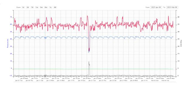
The Red/Pink axis represents the GCCC supply pressure. The Blue axis represents the supply pressure to the Sanctuary Cove site from the PRVs. Please refer to below graphs/data illustrating significant fluctuations in the incoming supply pressure from GCCC compared to the current supply pressures at Sanctuary Cove.
