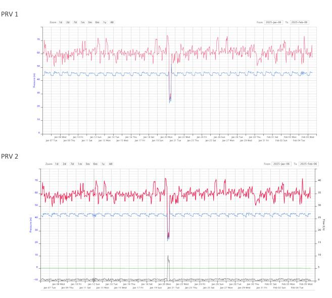
The Red/Pink axis represents the GCCC supply pressure. The Blue axis represents the supply pressure to the Sanctuary Cove site from the PRVs. Please refer to below graphs/data illustrating significant fluctuations in the incoming supply pressure from GCCC compared to the current supply pressures at Sanctuary Cove.
