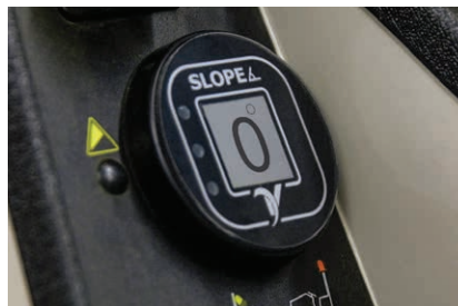
Digital Slope Gauge Recommended for operation on slopes.
