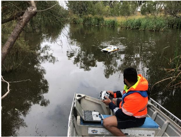
Left: Accura being operated from powered dinghy (Chinchilla River), Right: Data display on Hypack
